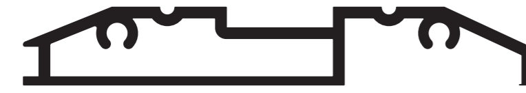
SD501 DRAINED THRESHOLD
